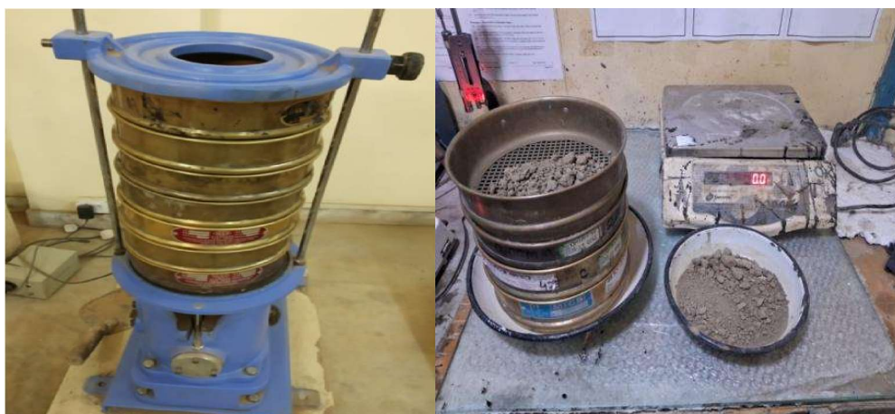
Fig.1 Instrument used in the study (a) Sieve Shaker (b) Set of Sieve
